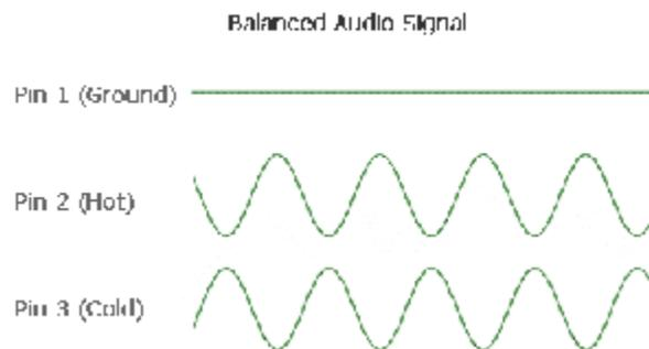
Notice that our signals look exactly the same, but they are offset in time with each other by 180 degrees – as one sine wave is on the way up, the other is on the way down.
