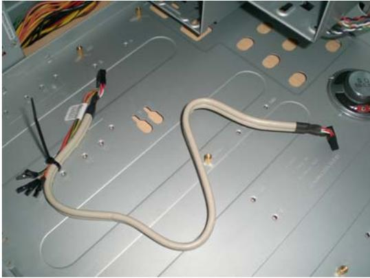
This is the USB cable in its unplugged state. Note the wire tie securing the little wires on the motherboard end. The OTHER end plugs into the front panel.
