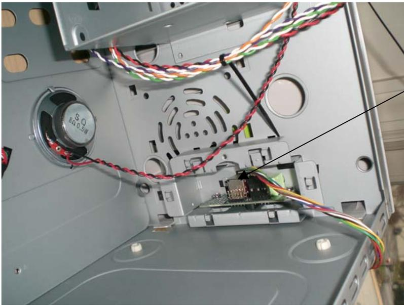
You are going to plug it in here. Note how one pin is missing – this is the “key” so you can only plug it in one way.
