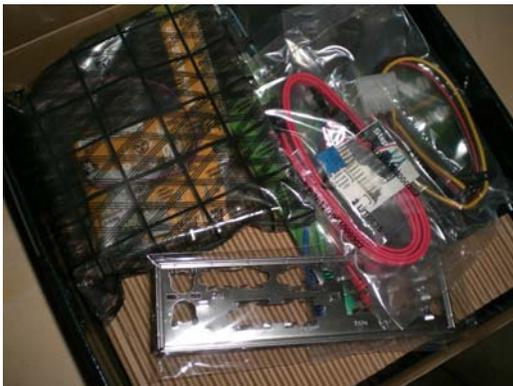
This is easy to install once you done it a few times. What? You have never done it? Ok then, just follow along and we'll show you how. **First, orient the metal panel and note how to the edges have a bit of spring to them. Place the panel inside the opening FROM THE INSIDE of the case like you see here.**
