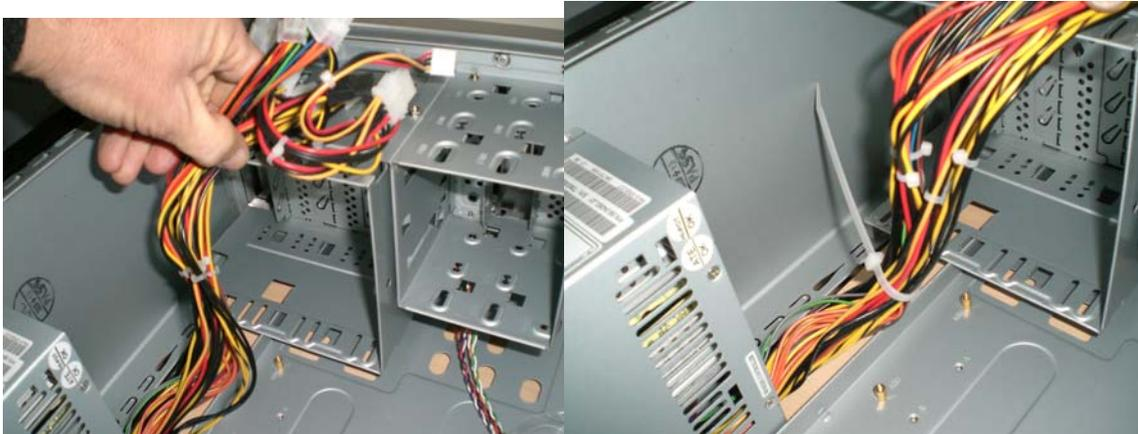
Also drape the case fan power cable over the side. When you are done with that, **remove the rubber band from the bundle of small wires that come from the front panel of the case.** These go to the various lights and switches on the front panel. **Do NOT keep the speaker cable in this bundle. Just let it stay separate from the others.**
