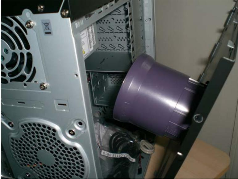
Inside the case are some giblets we need to remove. In this case, our giblets are the power cord and the pack that contains the instructions for the case and the package of screws. **Set aside the power cord and open the package of screws and dump the whole load into our screw bowl.**
