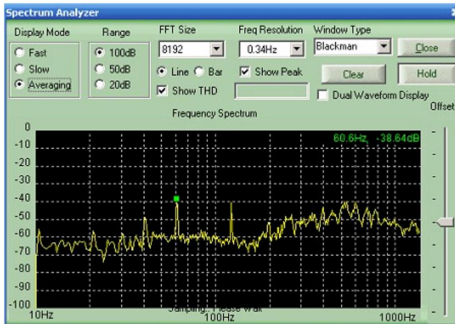
Notice the two hum signals - one at 60hz and another at 120hz. Aha! This is why our Ezclean only got half the hum - it works on Odd harmonics (which would be 60 and 180hz), while this is the more unusual even harmonics - 60 and 120hz.
